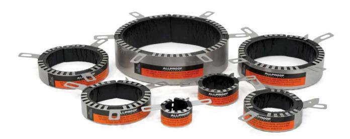
The low profile fire collars are designed to be installed in concrete, masonry fire rated walls and floors, and fire rated plasterboard walls. The Allproof fire collars consist of intumescent material encased in a steel surround with fixing tabs. The advanced intumescent technology allows Allproof to achieve a very low profile height of only 28mm.
